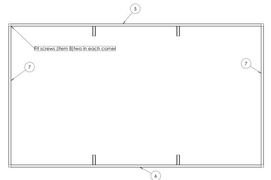
5. Next insert the two remaining tubes (7) into the metal saddle brackets using the colour coded dots to get them in the correct position. The tubes slide into the saddle clamps as shown below.
