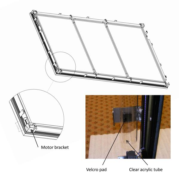
7. With The screen still lying flat on the ground, route the cord from the counter-weight carefully over the small white pulley above the top of the clear tube. Apply a little tension and ensure that the cord is taking the most suitable and direct route to and from the counter-weight. The lower end of the cord is attached to the end of the lower mask.
