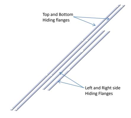
First, with two people, turn the subframe assembly up-side down on the floor so that the white fabric is on your clean plastic sheet. Next, using the colour coding, mate the internal hiding flanges with the colour coding dots on the upper surface of the sub-frame assembly. The holes are pre-drilled. The hiding flanges are then screwed in position using the self threading screws provided. The diagram below shows how the hiding flanges fit relative to the subframe, the grip fix and the material.
