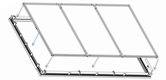
5. The subframe is fixed to the main frame using 6 M6 screws. The diagrams below show their locations.
