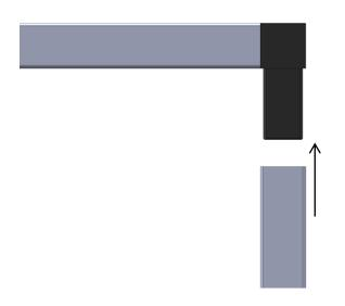
4. Now fit the self threading screws (8) into the pre-drilled holes to fix the vertical sections to the plastic corner pieces. DO NOT TRY TO MOVE THE SUBFRAME AT THIS POINT.
