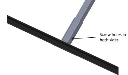
6. Now fit the self threading screws (8) into the pre-drilled holes to fix the vertical sections to the metal saddle clamps.
