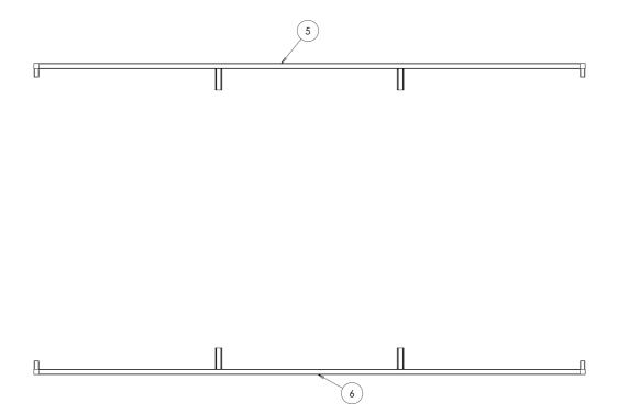
3. Next insert the two side tubes (7) using the colour coded dots to get them in the correct position. The tubes slide over the plastic end pieces on items (5) and (6).
