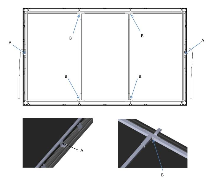
6. With The screen still lying flat on the ground, working on one side at a time, carefully lower the cylindrical counter-weight into the top of the clear acrylic tube until it is almost fully inside.
