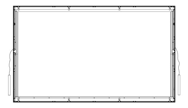
4. The next stage is to fit the subframe to the main frame. The subframe is marked TOP and must be presented to the main frame in the correct orientation.
