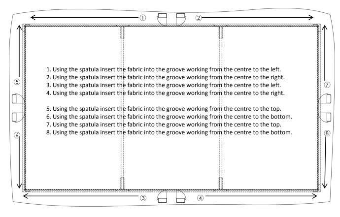
9. Once the material is neatly fitted into the GripFix profile and the projection surface is free of wrinkles, with a pair of sharp scissors neatly and carefully trim the excess black and white material so that it is flush with the outside of the sub-frame.
