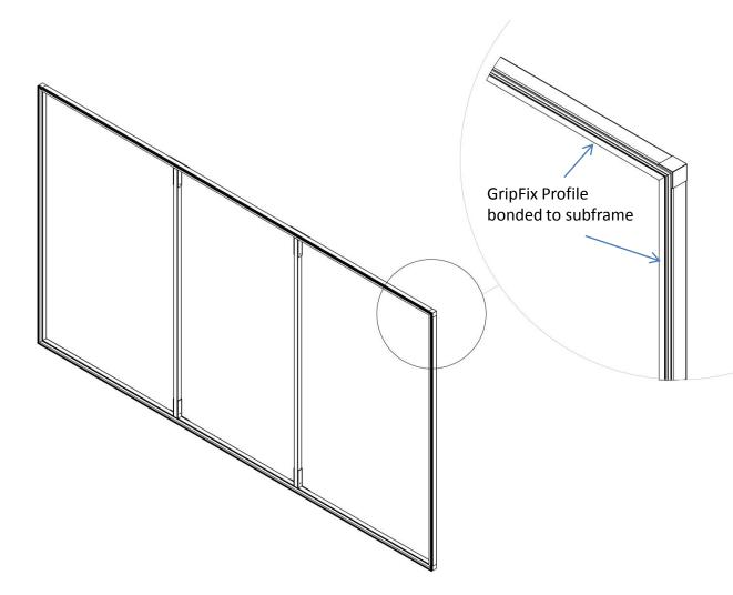
7. It is now time to fit the black backing material. Remove the black material from its bag, unfold it and lay it over the finished subframe. The material is larger than the subframe. Using the plastic spatula supplied follow the sequence as shown below to insert the fabric into the GripFix profile. Try to get the material taut and wrinkle free. Try a rolling action with the spatula to aid fitting.
