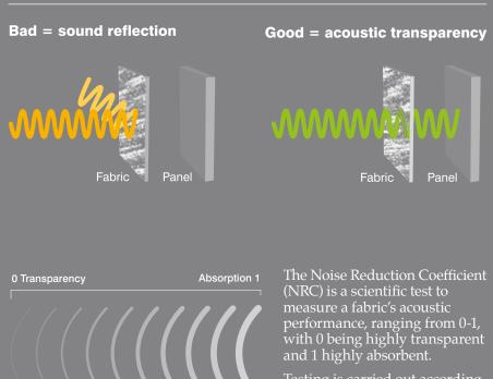
Testing is carried out according to the British Standard BS EN ISO 10534, (2001).
