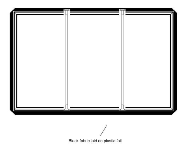
Note: On the drawing the 2 stiffening bars have been represented as for a 100" or over base width
