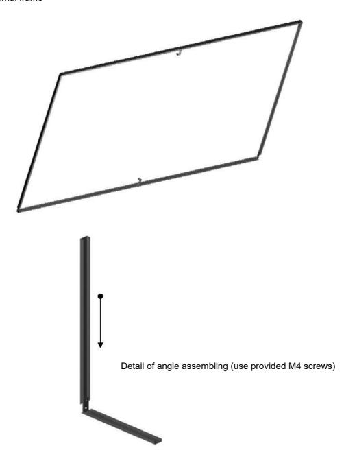
Assemble the external frame around the main frame.
