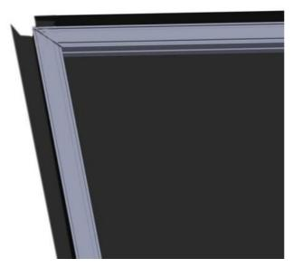
Place provided pi-grip/grip-fix on fabric laying on frame. Using supplied mallet, insert the Black Backing into the groove on the rear face of the frame, trapping the fabric in the groove. The action of pushing the fabric will tension it. Again, ensure that the fabric is smooth and wrinkle free. Do it around frame.
