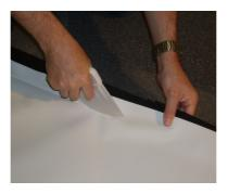
Once you have fitted the white fabric, turn the screen over and carefully inspect the screen surface to ensure that you are happy with the tension and the smoothness of the surface.
